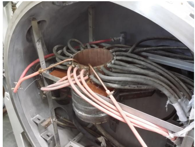
Fig. 2: Design of cold crucible for continuous pouring
