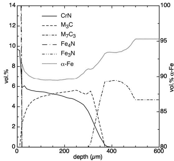
Fig. 2: Volume fraction-depth profiles of each phase. Thermo-Calc calculations.
