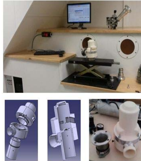
Fig. 3. Wind tunnel and experimental cylinder.
