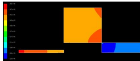
Fig. 8. Pressure field (in bar) at \theta=245 CAD.
