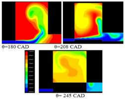
Fig. 12. Mass fraction of burnt gases.
