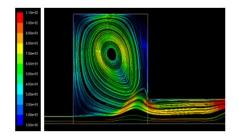
Fig. 9. Velocity pathlines(in m/s) at  $\theta$ =180 CAD.
