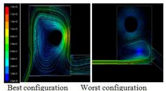
Fig. 14. Mass fraction of burnt gases at  $\theta$ =180 CAD.
