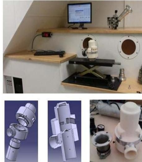
Fig. 3. Wind tunnel and experimental cylinder.
