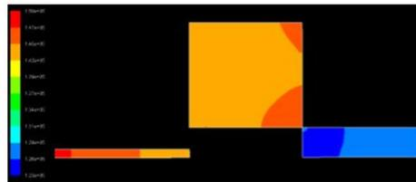
Fig. 8. Pressure field (in bar) at  $\theta=245$  CAD.
