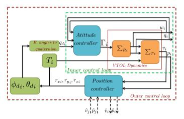
Fig. 3. Block diagram of the even-based control strategy
