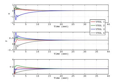
Fig. 10. Linear velocity vectors,  $(v_{x_i}, v_{y_i}, v_{z_i})$  m/s.
