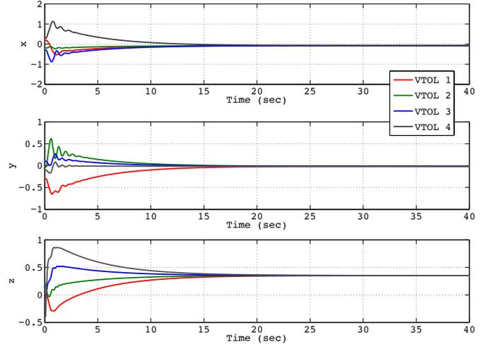
Fig. 7. Linear velocity vectors,  $(v_{x_i}, v_{y_i}, v_{z_i})$  m/s.
