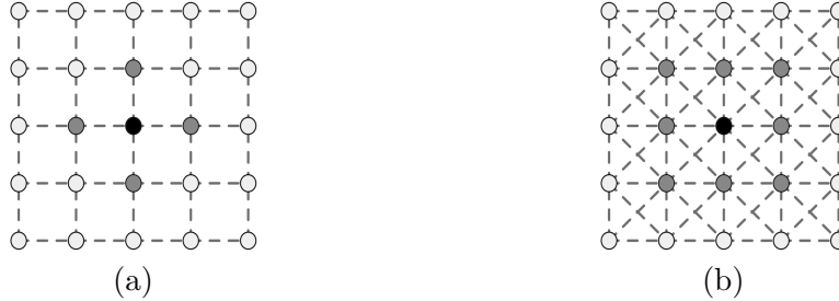
Figure 1: Neighborhood graphs \mathcal{G} of hidden Potts model. (a) The four closest neighbour graph \mathcal{G}_4 defining model \text{HPM}(\mathcal{G}_4, \theta, K) . (b) The eight closest neighbour graph \mathcal{G}_8 defining model \text{HPM}(\mathcal{G}_8, \theta, K) .
