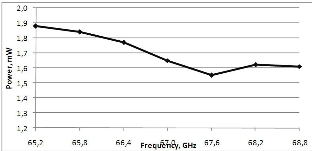
Figure 2 – Graph of dependency of signal power on frequency in the frequency range from 65.2 GHz to 68.8 GHz with a step of 0.6 GHz at the output of the measuring channel. The signal power at the output of the generator is 3,62mW .
