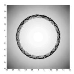
Fig. 11.4. Numerical precession and nutations projected on the (x, y)-plane for  $t \in [0, 100]$  of the axis of a heavy top. The equations are solved in body coordinates (employing the coadjoint action) with the Lie-group scheme RKMK4.
