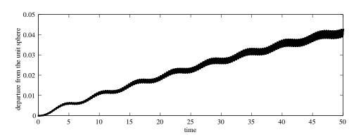
Fig. 11.3. Departure from unity for 'unit vector' along the axis of the top for  $t \in [0, 100]$ . The equations are solved in body coordinates with the MATLAB routine ode45.
