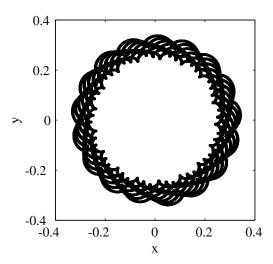
Fig. 11.2. Numerical precession and nutations projected on the (x, y)-plane for  $t \in [0, 100]$  of the axis of a heavy top. The equations are solved in body coordinates with the MATLAB routine ode45.
