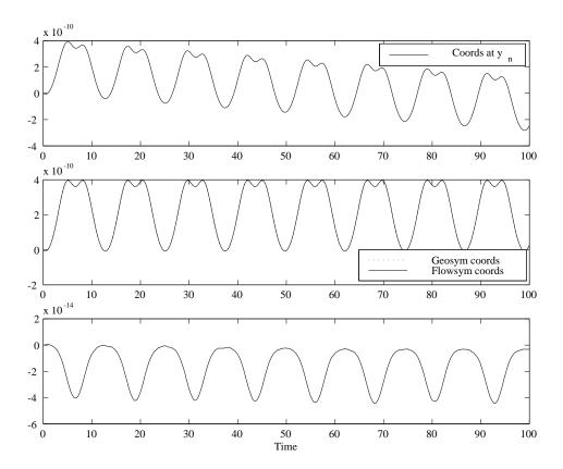
Fig. 7.2. Error in the Hamiltonian versus time for an order-four RK-MK method based on Gaussian nodes. The top plot corresponds to coordinates centred at  $\boldsymbol{y}_n$  while the second plot corresponds to geodesic and flow-symmetric coordinates. Although generally the two latter choices would correspond to different error, in this case the errors are very similar. The bottom plot corresponds to the difference between the errors in geodesic and flow-symmetric coordinates.
