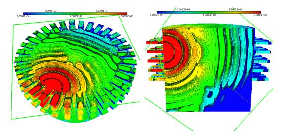
Figure 5: Slices showing the norm of the real part of the total field  $\mathbf{E}$  in the imaging chamber with the plastic-filled cylinder inside, for a transmitting antenna in the second ring from the top.
