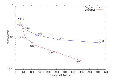
Figure 6: Time to solution (seconds) and relative error on the computed  $S_{ij}$  with respect to the reference solution, using edge finite elements of degree 1 and degree 2 for different mesh sizes. The total number of unknowns in millions is also reported for each simulation.
