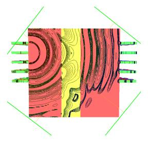
Figure 4: Slice of the imaging chamber, showing the non-dissipative plastic-filled cylinder and some isolines of the norm of the real part of the total field  $\mathbf{E}$ .
