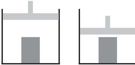
FIGURE 1 Schematical representation of the porosimeter. The sample is contained in a closed cell and volume is changed using a moveable piston. In practice, the volume changes are extremely small.
