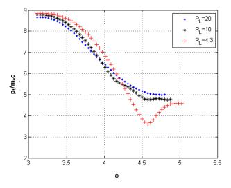
FIG. 6. Final electron momentum  $p_f/(mc)$  as a function of the entry phase in the surface plasma wave field going from  $R_L=4.3$  ( $\omega/\omega_{pe}=0.22$ ) to  $R_L=20$  ( $\omega/\omega_{pe}=0.05$ ). Only the electrons in the vacuum side have been considered.
