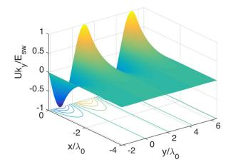
FIG. 10. Electrostatic potential [Eq. (11)] as a function of space for the case  $R_L = 4.3 \ (\gamma_{\phi} = 4.54, \ \omega/\omega_{pe} = 0.22, \ \phi = 0)$ .
