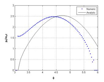
FIG. 4. Final electron momentum  $p_f/(mc)$  as a function of the entry phase in the surface plasma wave field for  $R_L=0.2$  ( $\omega=0.7\omega_{pe}$ ) (the black full line is the analytic prediction Eq. (8)). Only the electrons in the vacuum side have been considered.
