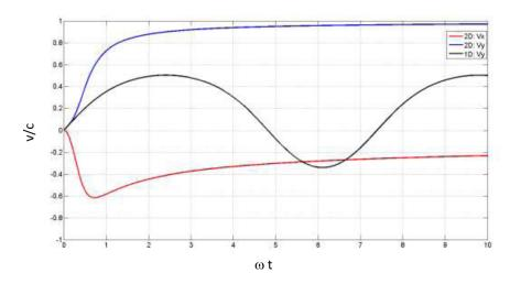
FIG. 9. Evolution of the normalized electron velocity with time for the entry phase  $\phi=3.14$  in the surface plasma wave field within the relativistic electromagnetic regime for  $R_L=20$  ( $\gamma_{\varphi}=20$  and  $\omega/\omega_{pe}=0.05$ ):  $v_x$ ,  $v_y$  (2D simulation), and  $v_y$  (setting  $E_x=B_z=0$ ). Only the electrons in the vacuum side have been considered.
