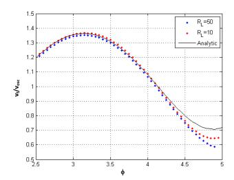
FIG. 1. Non-relativistic limit: final electron velocity  $v_f/v_{osc}$  as a function of the entry phase  $\phi$  in the SPW field. Here,  $\frac{1}{2}mv_0^2=100\,\mathrm{eV}$  and  $v_{osc}/c\sim a_{sw}=0.086$ . We plot Eq. (6) (the black full line), and the numerical values for  $R_L\sim 50~(\omega=0.22\omega_{pe})$  (the blue diamond), and  $R_L\sim 10~(\omega=0.6\omega_{pe})$  (the red diamond). Only the electrons in the vacuum side have been considered.
