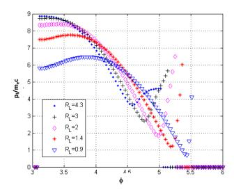
FIG. 5. Final electron momentum  $p_f/(mc)$  as a function of the entry phase in the surface plasma wave field. Various values of  $\omega/\omega_{pe}$  are considered. By varying this parameter, we explore the values from  $R_L=4.3$  ( $\omega/\omega_{pe}=0.22$ ) to  $R_L=0.9$  ( $\omega/\omega_{pe}=0.6$ ), where the latter value tends towards the electrostatic regime. Only the electrons in the vacuum side have been considered.
