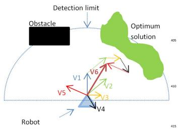
Figure 1: Robot position's updating
