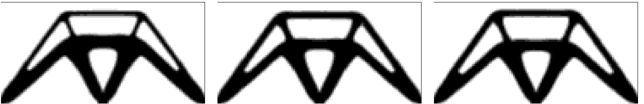
Figure 18: Final domains for the gradient algorithm on problem of Section 7.3.4. From left to right, gradient with extension 4.3, gradient with extension 4.1, gradient with extension 4.2.
