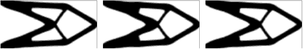
Figure 36: Final domains for Newton's algorithm on problem of Section 7.4.2. From left to right, Newton with extension 4.3, Newton with extension 4.1, Newton with extension 4.2.
