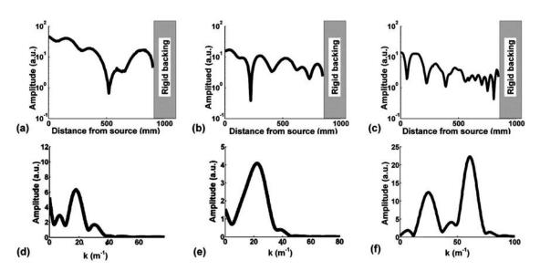
FIG. 4. (a), (b), and (c): Experimental standing wave patterns. (d), (e), and (f): Spatial Fourier transforms of the measured standing wave patterns. (a) and (d) 256 Hz; (b) and (e) 424 Hz; (c) and (f) 1041 Hz.
