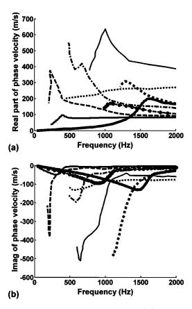
FIG. 5. Dispersion curves calculated by solving Eq. (30) numerically for a melamine foam of 0.1-m thickness. (a) Real part and (b) imaginary part of the phase velocities. The anomalous behavior of the dashed-curve mode around 250 Hz is due to numerical error.
