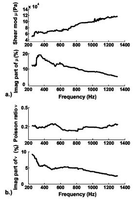
FIG. 9. Fitted real and imaginary parts of the shear modulus and Poisson ratio against frequency. The imaginary parts are plotted in percentage of the real parts.
