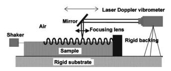
FIG. 3. Experimental setup for the generation and detection of standing waves in a layer of material on a rigid substrate.
