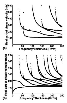
FIG. 2. Phase velocities vs frequency×thickness for (a) a plate of thickness H of an elastic material on a rigid substrate; (b) a Lamb plate of thickness 2H. In both cases the material density is  $14 \text{ kg/m}^3$ ,  $V_L = 222 \text{ m/s}$ , and  $V_T = 122 \text{ m/s}$ .
