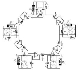
Fig. 8 Five identical coupled Chua's circuits forming a ring<sup>[13]</sup>
