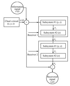
Fig. 18 Block diagram of the electronic circuit implemented in Fig. 19
