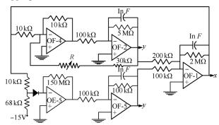
Fig. 5 Electronic circuit representation of a modified Rössler's  $\operatorname{system}^{[9]}$
