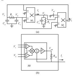
Fig. 4 Lorenz's circuit. (a) Schematic diagram of a simple circuit. Analog multipliers  $M_1$  and  $M_2$  are configured as current output devices; (b) Schematic diagram of a generic analog multiplier  $M_i$  configured as a current output device<sup>[8]</sup>
