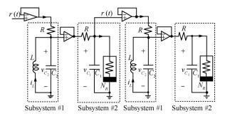
Fig. 19 Electronic circuit implementation of the two-stage "receiver" consisting of two identical copies of the circuit given in
