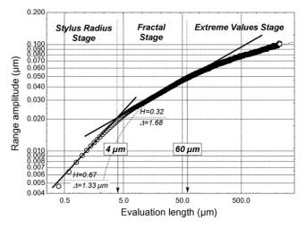
Fig. 3.  $R_l(l)$  multi-scale mean roughness values at different observation scales l obtained by averaging the nine recorded aluminium surface profiles tooled with HPT shown in Fig. 2.
