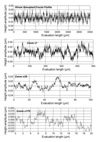
Fig. 6. Simulated profile of surface tooled with HPT as shown in Fig. 1 with three spatial zoom (X7, X35, X175) located at the origin of the whole profile.
