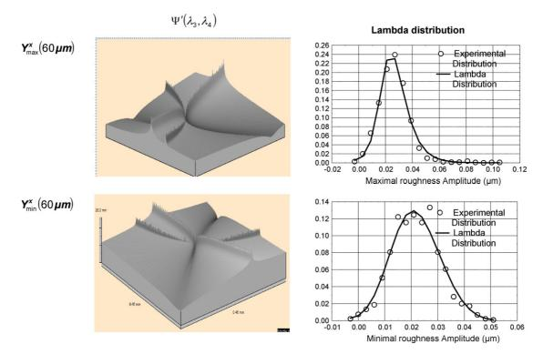
Fig. 10. 3D view of the values of the function  $\Psi(\lambda_3,\lambda_4)$  for the lambda distribution associated with  $Y^x_{max}$  (60 µm) and  $Y^x_{min}$  (60 µm). On the right,  $Y^x_{max}$  (60 µm) and  $Y^x_{min}$  (60 µm) Lambda distribution obtained after minimization on  $\Psi(\lambda_3,\lambda_4)$ .
