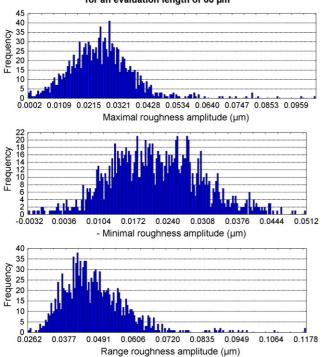
Fig. 9. Minimal  $Y_{min}(l)$ , maximal  $Y_{max}(l)$ , and range roughness amplitude  $R_t(l)$  empirical distributions at  $l = 60 \,\mu\text{m}$  evaluation scale.
