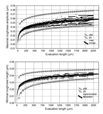
Fig. 12. Prevision of the mean of the extreme roughness amplitude parameters  $\hat{Y}_{max}^{60\,\mu m,k}$ ,  $\hat{Y}_{min}^{60\,\mu m,k}$  ( $\blacktriangle$ ) vs. the evaluation length (obtained by taking all *k* values) and their associated 5th ( $\bigcirc$ ) and 95th ( $\Box$ ) quantile confidence intervals. The 9 experimental curves are plotted ( $\diamondsuit$ ).
