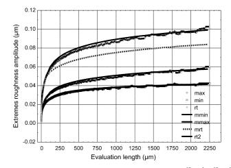
Fig. 13. Mean of the extreme roughness amplitude parameters  $\hat{Y}_{max}^{60\,\mu m,k}$ ,  $\hat{Y}_{min}^{60\,\mu m,k}$ ,  $\hat{R}_{t}^{60\,\mu m,k}$  and  $\hat{R}_{t2}^{60\,\mu m,k} = \hat{Y}_{max}^{60\,\mu m,k} - \hat{Y}_{min}^{60\,\mu m,k}$  (lines) prevision vs. the evaluation length and the  $Y_{max}(l)$ ,  $Y_{min}(l)$  and  $R_{t}(l)$  means experimental values.
