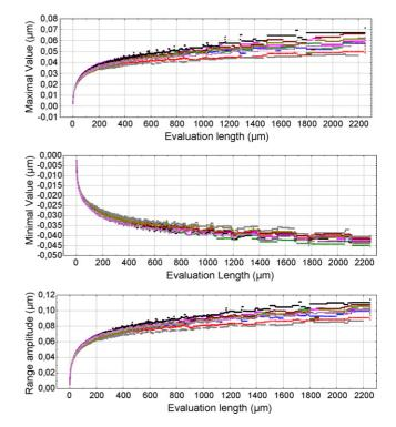
Fig. 2.  $Y_{\text{max}}(l)$ ,  $Y_{\text{min}}(l)$  and  $R_t(l)$  multi-scale roughness values at different observation scales *l* for nine recorded aluminium surface profiles tooled with HPT.
