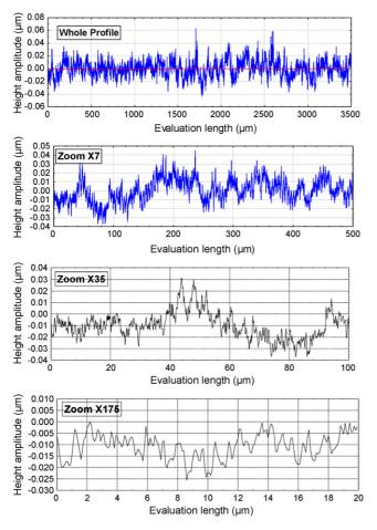
Fig. 1. Recorded profile of an aluminium surface tooled with HPT with three spatial zoom (X7, X35, X175) located at the origin of the whole profile.
