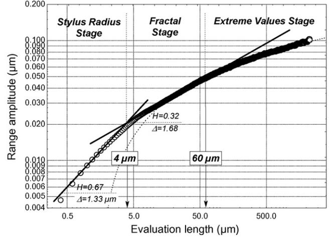
Fig. 3.  $R_t(l)$  multi-scale mean roughness values at different observation scales  $l$  obtained by averaging the nine recorded aluminium surface profiles tooled with HPT shown in Fig. 2.
