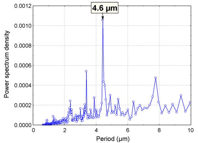
Fig. 5. Average power spectrum of the nine aluminium surface recorded profiles tooled with HPT.
