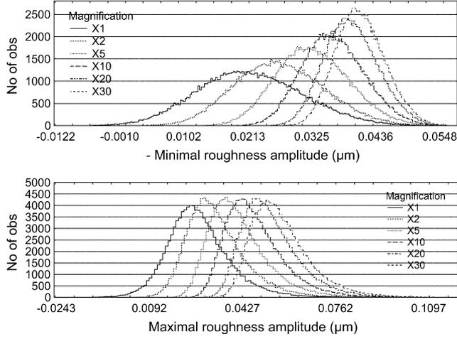
Fig. 11.  $\hat{Y}_{\max}^{60\mu\text{m},k}$  (top) and  $\hat{Y}_{\min}^{60\mu\text{m},k}$  (bottom) PDF's functions prediction obtained from 10000 Monte-Carlo simulations for the 6 magnifications  $k \in \{1,2,5,10,20,30\}$ . The case  $k=1$  corresponds to simulation of the original Lambda shown on Fig. 10.
