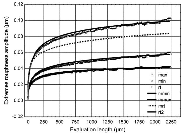
Fig. 13. Mean of the extreme roughness amplitude parameters  $\hat{Y}_{\max}^{60\mu\text{m},k}$ ,  $\hat{Y}_{\min}^{60\mu\text{m},k}$ ,  $\hat{R}_t^{60\mu\text{m},k}$  and  $\hat{R}_{t2}^{60\mu\text{m},k} = \hat{Y}_{\max}^{60\mu\text{m},k} - \hat{Y}_{\min}^{60\mu\text{m},k}$  (lines) prevision vs. the evaluation length and the  $Y_{\max}(l)$ ,  $Y_{\min}(l)$  and  $R_t(l)$  means experimental values.
