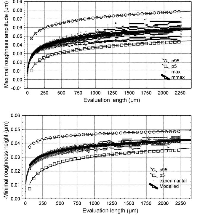
Fig. 12. Prevision of the mean of the extreme roughness amplitude parameters  $\hat{Y}_{\max}^{60\mu\text{m},k}$ ,  $\hat{Y}_{\min}^{60\mu\text{m},k}$  ( $\blacktriangle$ ) vs. the evaluation length (obtained by taking all  $k$  values) and their associated 5th ( $\circ$ ) and 95th ( $\square$ ) quantile confidence intervals. The 9 experimental curves are plotted ( $\diamond$ ).
