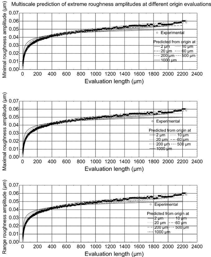
Fig. 15. Multi-scale prediction of extreme roughness amplitudes parameters  $\hat{Y}_{\min}^{x,k}$ ,  $\hat{Y}_{\max}^{x,k}$ ,  $\hat{R}_t^{x,k}$  at different origin evaluations  $x \in \{2, 10, 20, 60, 200, 500, 1000\}$ .
