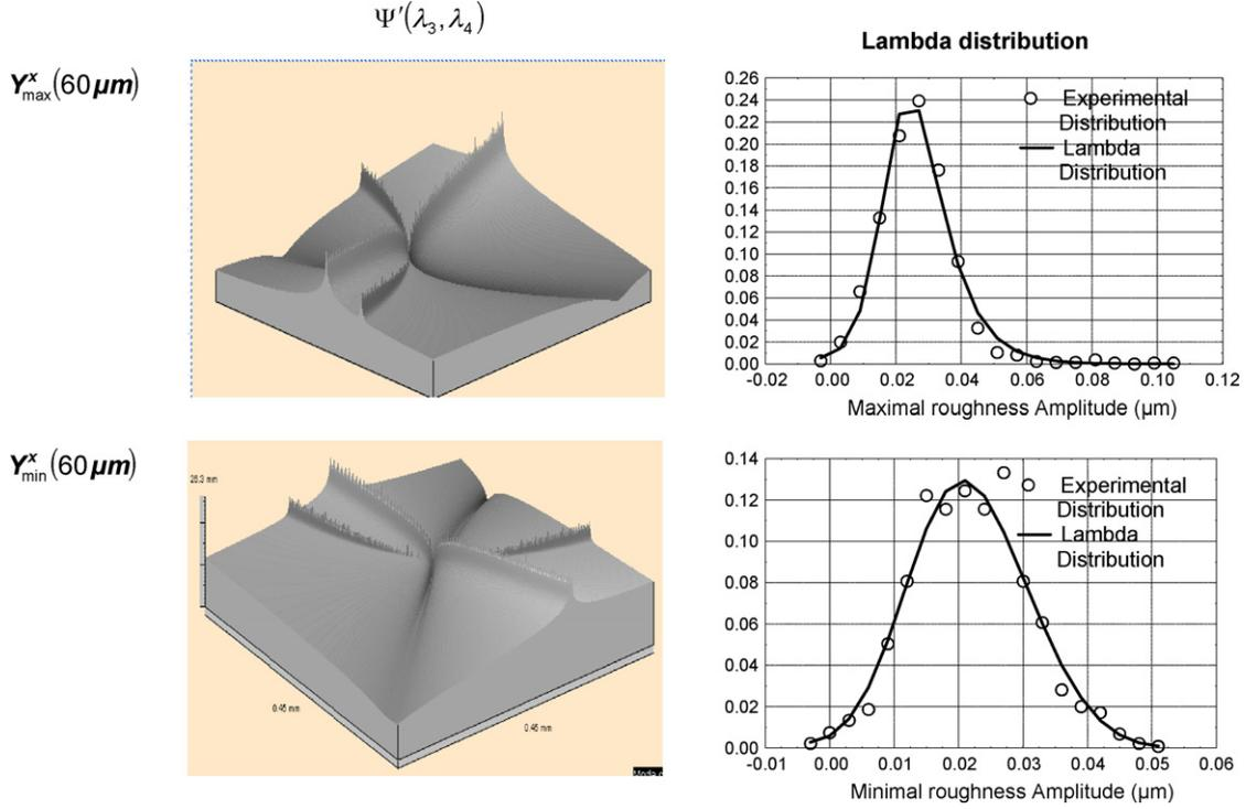
Fig. 10. 3D view of the values of the function  $\Psi(\lambda_3, \lambda_4)$  for the lambda distribution associated with  $Y_{\max}^x(60 \mu\text{m})$  and  $Y_{\min}^x(60 \mu\text{m})$ . On the right,  $Y_{\max}^x(60 \mu\text{m})$  and  $Y_{\min}^x(60 \mu\text{m})$  Lambda distribution obtained after minimization on  $\Psi(\lambda_3, \lambda_4)$ .
