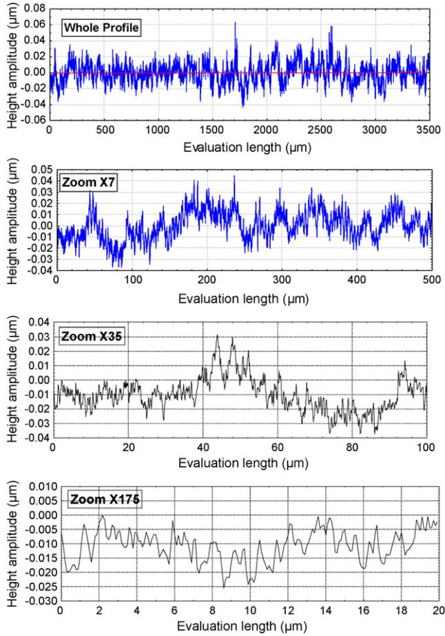
Fig. 1. Recorded profile of an aluminium surface toolled with HPT with three spatial zoom (X7, X35, X175) located at the origin of the whole profile.
