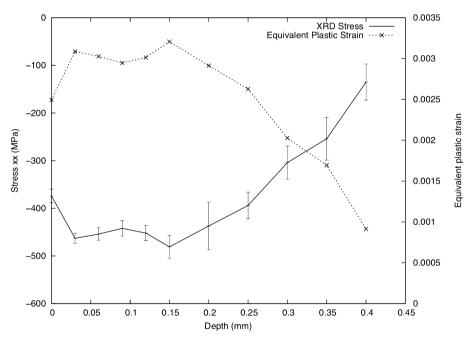
Fig. 9. Shot peened specimen with an Almen intensity of F51A and a coverage ratio of 110% using 0.6 mm diameter shot. Residual stresses determined by X-ray diffraction. Corresponding plastic strains (Eq. (3)).
