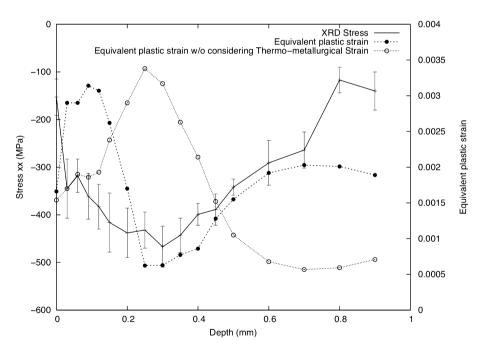
Fig. 14. Experimental residual stress profiles of carbonitrided 29MnCr5 Steel. Calculated equivalent plastic strain with and without considering thermometallurgical strains.
