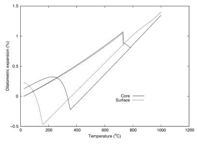
Fig. 12. Dilatometric expansion curves obtained with JMatPro. 29MnCr5 steel grade with a composition of 0.29%wt C in the core of the material and 0.85%wt C – 0.3%wt N near the surface.
