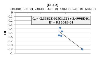
Fig. 5. Example  $C_0 = g(C_1, C_2)$  using experimental data. Each point corresponds to a result extracted from experimental data [33].
