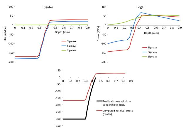
**Fig. 19.** Top: residual stress profiles as a function of the depth along the red lines represented in Fig. 11 and taken at the center of the tooth and close to its edge. Bottom: comparison of the residual stress field obtained in the middle of the tooth and the one obtained in a semi-infinite body treated with the same conditions as the gear.
