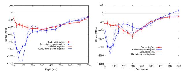
Fig. 16. Stress profiles after carburizing and after shot peening and after carbonitriding followed by shot peening – Experimental data obtained by XRD (solid lines) and results of finite element calculation (dashed lines).
