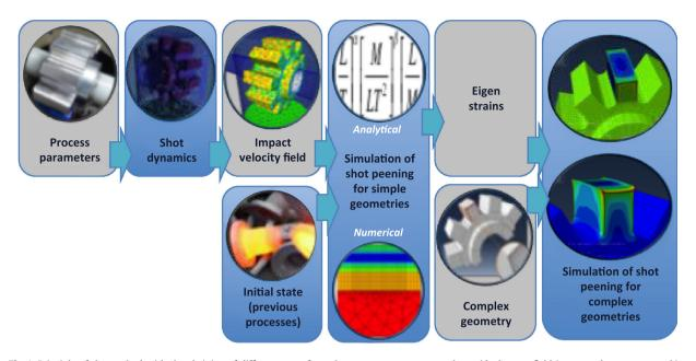
Fig. 1. Principle of the method with the chaining of different steps from the process parameters to the residual stress field in a complex geometry taking into account an initial state coming from previous manufacturing processes.
