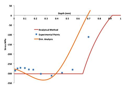
**Fig. 6.** Residual stress in a shot-peened rod made of aluminum (yield stress  $\sigma_y = 310$  MPa and hardening slope h = 1200 MPa). The models correspond to the dimensional analysis presented in Section 4.1 (orange line) and to the analytical model presented in Section 4.2 (red line). The experimental data is presented with blue squares [36]. The shot peening parameters are V = 80 m/s for the shot velocity and R = 0.45 mm for the steel shot radius.
