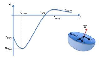
Fig. 2. Typical residual stress profile induced by shot peening.
