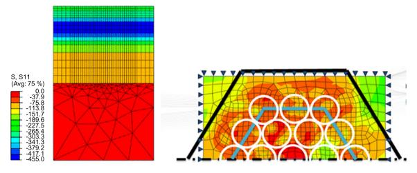
Fig. 15. Induced stress after carburizing (left) and shot peening finite element model with 12 spheres on a symmetric semi-infinite body (right).
