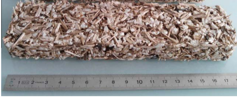
Fig. 1. A sample of sunflower stem/chitosan bio-based composite.
