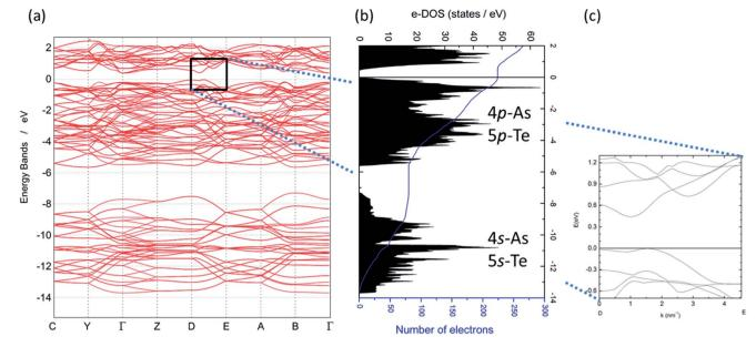
**Fig. 2** Electronic structure of the  $\beta'$ -As<sub>2</sub>Te<sub>3</sub> phase: (a) dispersion curves along high symmetry directions represented in the irreducible  $P2_1/m$ Brillouin zone and (b) density of states (DOS) as a function of the energy. The Fermi level has been chosen as the origin of energies. (c) Magnification of the dispersion curves around the electronic band gap showing the four-top valence bands and the four top-most conduction bands.
