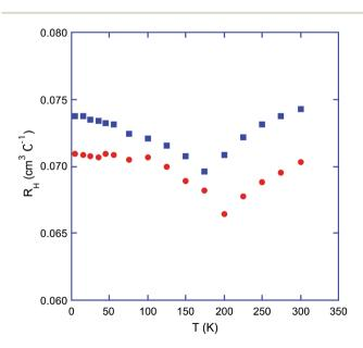
**Fig. 6** Hall coefficient  $R_{\rm H}$  as a function of the temperature measured parallel ( $\bullet$ ) and perpendicular ( $\blacksquare$ ) to the pressing direction.
