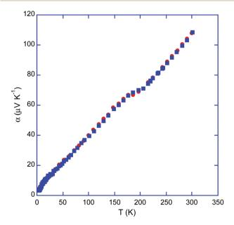
Fig. 7 Thermopower as a function of temperature of  $\beta$ -As<sub>2</sub>Te<sub>3</sub>. For sake of clarity, only the data collected in the parallel direction are shown. Measurement in the perpendicular direction yielded similar values and temperature dependences to within experimental uncertainty.
