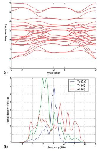
Fig. 3 (a) Phonon dispersion curves and (b) partial phonon DOS of the  $\beta'$ -As<sub>2</sub>Te<sub>3</sub> phase calculated in the irreducible C2/m Brillouin zone.
