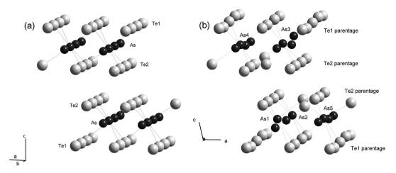
Fig. 1 Comparison of the rhombohedral (R3m) crystal structure (panel a) and the monoclinic ( $P2_1/m$ ) crystal structure (panel b) of the  $\beta$  and  $\beta'$  phases, respectively. Besides a slight distortion of the unit cell, a fourfold modulation of the atomic positions longitudinal and transverse to the *b* axis is observed in the  $\beta'$  phase. Both structures were drawn by using the experimental data obtained in ref. 29.
