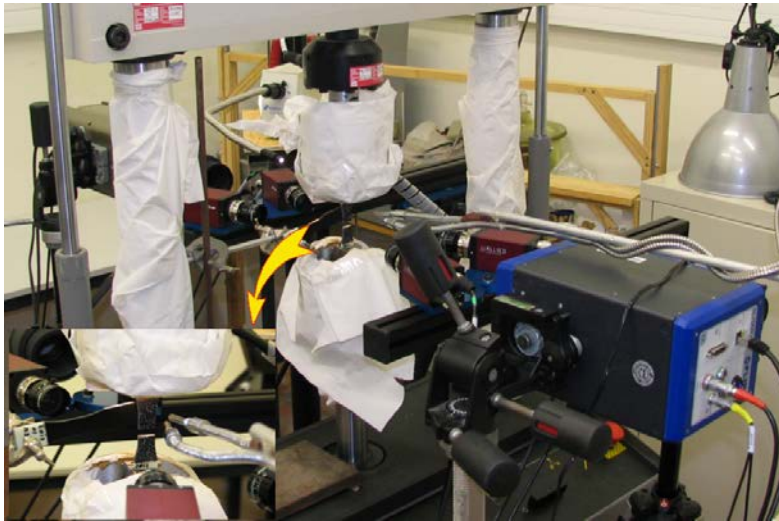
Fig. 3: Experimental setup showing both cameras used for recording the displacement and temperature fields.
