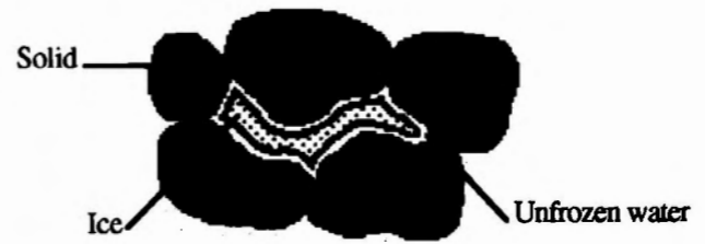
FIG. 1. Ice formation in frozen porous media.
