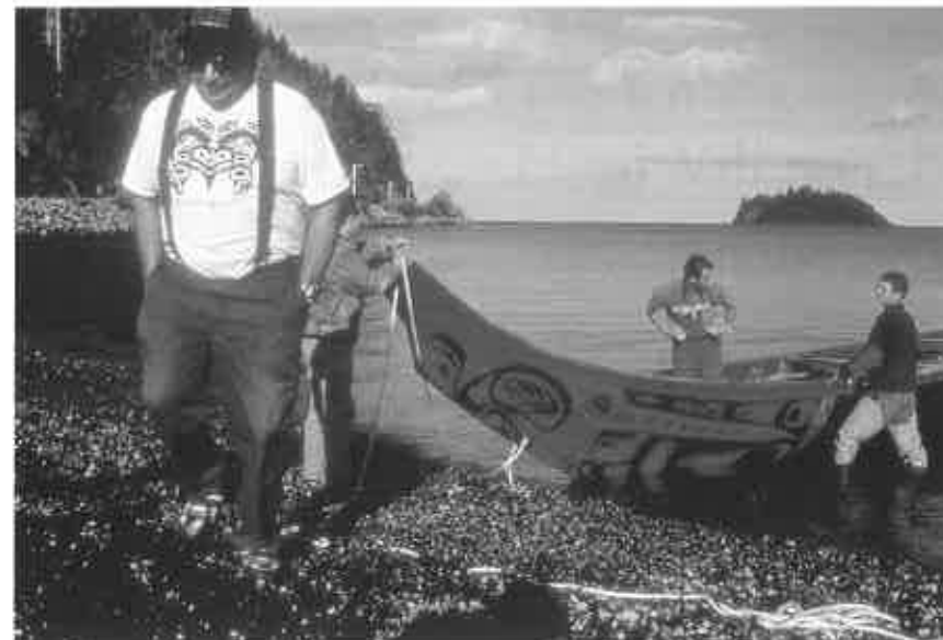
Fig. 5 The canoe named Lootas , carved out of a single cedar log according to traditional Haida techniques. Photograph: Michel Setboun/Planet.
