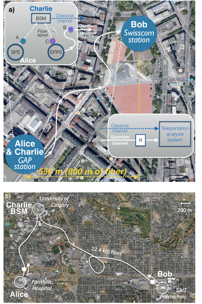
FIG. 3. Extending the reach. a) The 2007 Geneva teleportation experiment as an example in which photon B is already outside the lab when photon A is created, and continues to travel before being measured at Bob's [10]. b) The Calgary BSM as an example in which photons A and C are travelling a long distance before being jointly measured.
