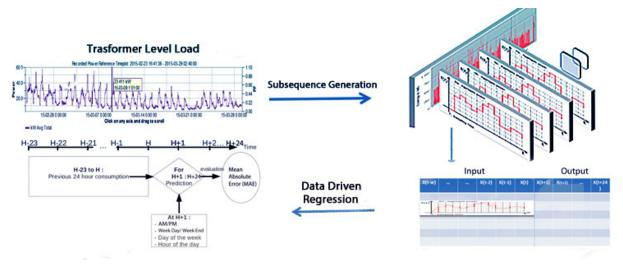
Fig. 3: Data representation in a standard propositional learning format.
