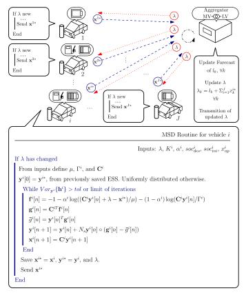
Fig. 1: Description of the decentralized MSD algorithm. With some important parameters as follow,  $\lambda$  is sum of total load and PEV distribution load;  $K^i$  is pure strategies,  $\alpha^i$  is trade-off parameter;  $soc_{ini}^i$  and  $soc_{des}^i$  are initial and desired states of charge of PEV respectively. All the other parameters can be referred to [4].
