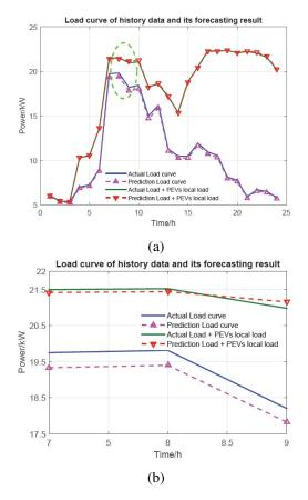
Fig. 6: Example of 24-hour optimization curves with actual history data and forecasting data, trade-off factor is set 0.95 and iteration times are equal to 50. Fig.6(a) is a zoom to part of Fig.6(b).
