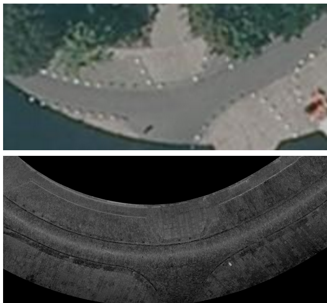
Figure 9: Comparison between aerial orthophotography with a standard resolution ( 50\text{cm}^2 per pixel) (top) and MLS orthoimage using our model at 1\text{cm}^2 per pixel (bottom). Traditional orthophotography provides limited resolution and suffers from occlusions brought by the coverage of trees and other structures whereas our model provides unobstructed, high resolution orthoimages. The aerial image comes from Geoportail.
