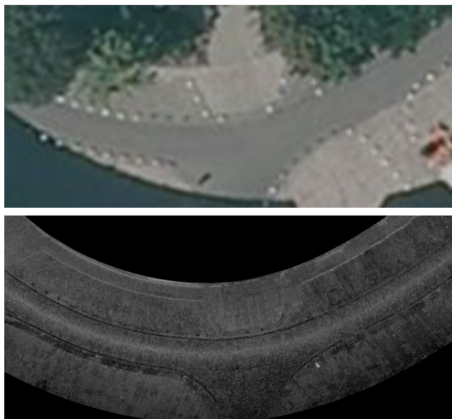
Figure 9: Comparison between aerial orthophotography with a standard resolution ( 50\text{cm}^2 per pixel) (top) and MLS orthoimage using our model at 1\text{cm}^2 per pixel (bottom). Traditional orthophotography provides limited resolution and suffers from occlusions brought by the coverage of trees and other structures whereas our model provides unobstructed, high resolution orthoimages. The aerial image comes from Geoportail.
