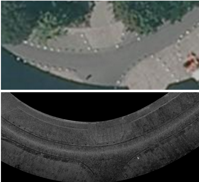
Figure 7: Comparison between aerial orthophotography (top) and MLS orthoimage (bottom). The MLS reconstruction contains \sim 6.10^6 px in which 72% were obtained by diffusion, and 10% by exemplar-based inpainting.
