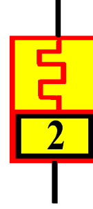
Fig. 3. Symbol of the second-order memristor.
