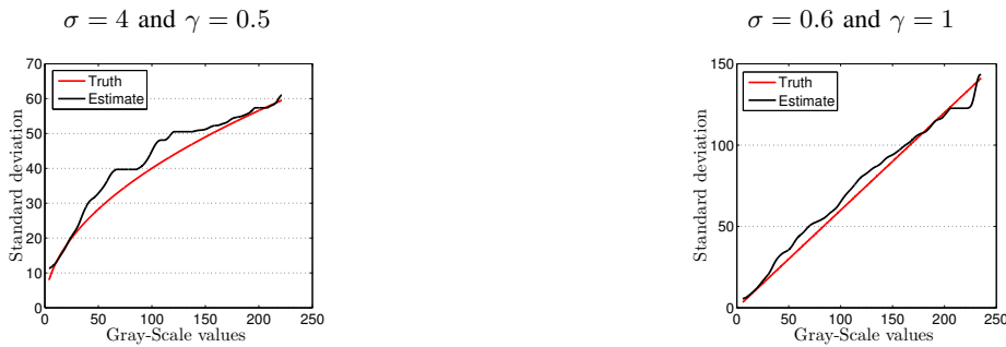
Figure 4: Standard deviation estimation from experiments on the “ Peppers ” image for different values of \sigma and \gamma .
