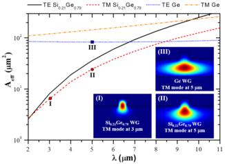
Figure: Effective modal area of fundamental TE and TM modes versus propagation wavelength for a  $Si_{1x}Ge_x$  waveguide (black straight line and red dashed line, respectively) and a Ge-on-Si waveguide (blue dotted line and orange dashed-dotted line). Insets I, II and III show the mode profile at selected wavelengths.
