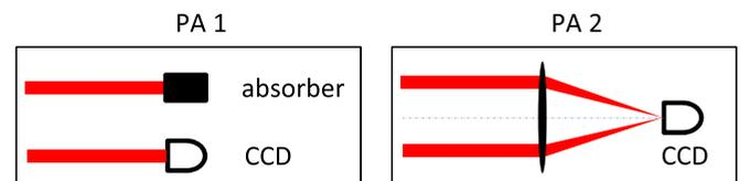
FIG. 4. Nonunitary gate (PA1) and parity analyzer (PA2).
