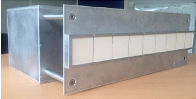
Fig. 2. Matrix antenna manufactured prototype.
