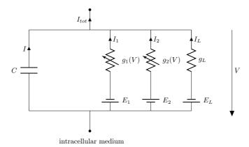
Figure 2 – Equivalent circuit for a conductance-based model with two types of channels
