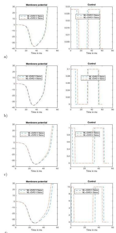
Figure 12 – Optimal trajectory and bang-bang optimal control for the ML-ChR2-3-states and ML-ChR2-4-states models with  $u_{max}=$  a) 0.028, b) 0.1, c) 1, d)  $10\,\mathrm{ms}^{-1}$ .
