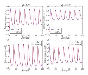
Figure 14 – Linear approximation of the variable h for a periodic behavior of system (HH) and initial membrane potential of -30, 0, 30 and 60 mV.
