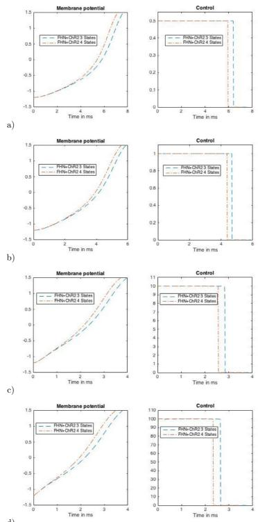
Figure 7 – Optimal trajectory and bang-bang optimal control for the FHN-ChR2-3-states and FHN-ChR2-4-states models with  $u_{max}=$  a) 0.5, b) 1, c) 10, d)  $100\,\mathrm{ms}^{-1}$ .
