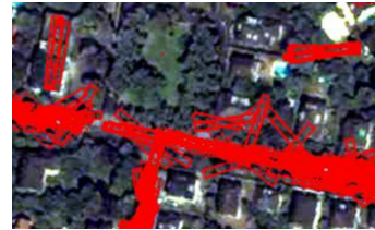
Fig. 3. Illustration of overlap among detected road segments (shown with red borders) to be corrected with the maximal overlapping ratio threshold.
