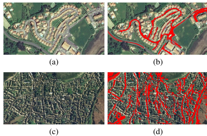
Fig. 15. Road network extraction on sample Pleiades images: (a) original image of St-Jean-de-Luz ©CNES 2013, Distribution Airbus DS and (b) extracted road network; (c) original image of Lorient ©CNES 2012, Distribution Airbus DS and (d) extracted road network.
