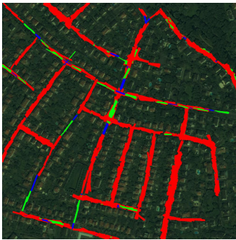
Fig. 9. Illustration of the ability of incomplete path filtering to reconnect disconnected road segments: initial segments are given in red, added segments are in blue, thus resulting in length updating in the path filtering process that is finally able to return new segments (in green).
