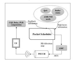
Fig. 4. Implemented model of the proposed scheduling scheme
