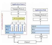
Fig. 1. Implemented model of VoLTE protocol stack used in LTE-Sim software
