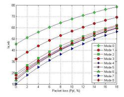
Fig. 3.  $I_{e,wb}$  vs.  $P_{pl}$  for nine modes of AMR-WB codec
