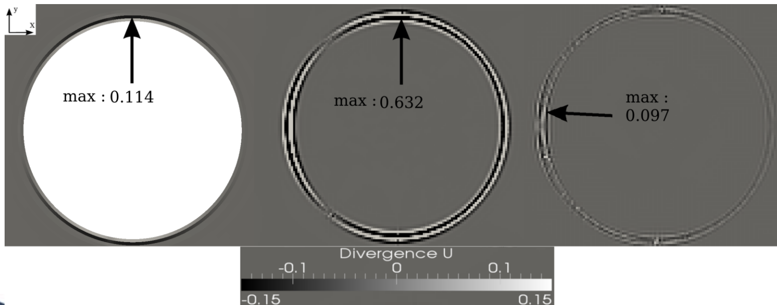
Plots of the velocity divergence around a 2D cylinder at Re = 30
