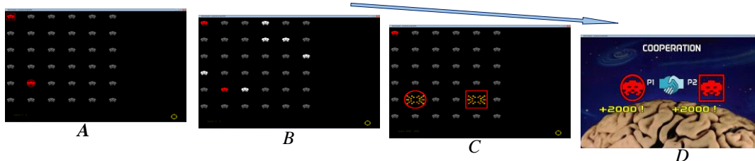
Figure 1. Brain Invaders v2: (A) Level initialization. (B) After a short delay, the game flashes randomly all the aliens. (C) The game destroys the most likely alien(s) according to the classification. (D) If the player(s) succeed(s) at destroying the target(s), s/he (they) is awarded by a fixed amount of points or by a factor proportional to the number of repetitions required.
