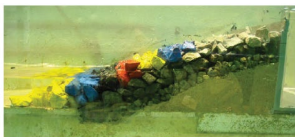
Figure 7 : Third layer with 5-6 T armour units and a 2 m raise of crown wall (a – left) and smoother slope of armour layer (1:3 slope instead of 1:2 slope) and a 1 m raise of crown wall (b – right).
