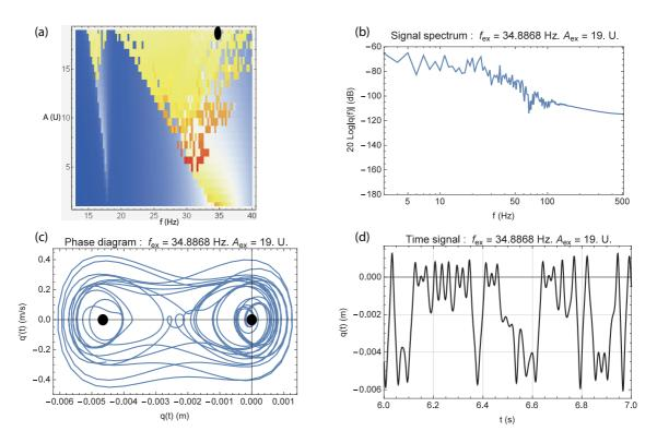
Figure 29: Computed BSA response. (a): density plot, the black oval represents the point of interest, (b): displacement spectrum, (c): phase plot, the black circles show the equilibrium points, (d): displacement time recording.
