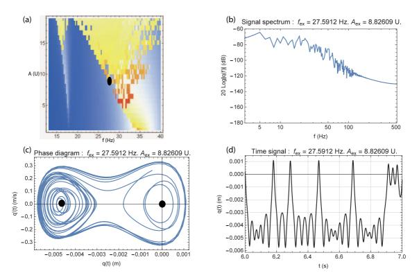
Figure 27: Computed BSA response.(a): density plot, the black oval represents the point of interest, (b): displacement spectrum, (c): phase plot, the black circles show the equilibrium points, (d): displacement time recording.
