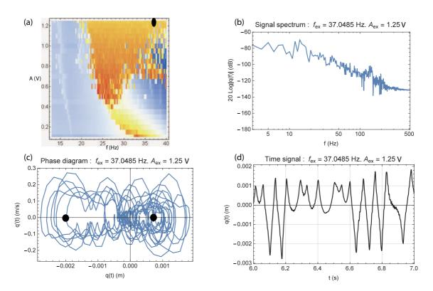
Figure 28: Measured BSA response. (a): density plot, the black oval represents the point of interest, (b): displacement spectrum, (c): phase plot, the black circles show the equilibrium points, (d): displacement time recording.
