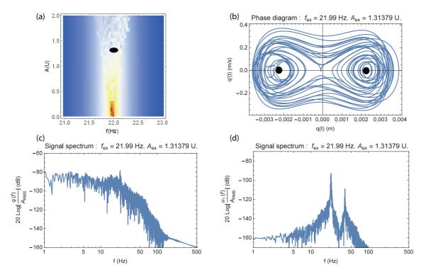
Figure 16: Typical calculated system response around the linear system first mode at an excitation frequency  $f_{ex} \approx 22$  Hz and amplitude  $A_{ex} \approx 1.31$  U. (a): density plot, the black oval represents the point of interest, (b): phase plot, the black circles show the equilibrium points, (c): BSA displacement spectrum, (d): beam 1 displacement spectrum.
