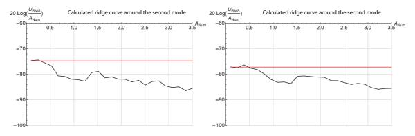
Figure 20: Calculated ridge curve of beam 1 displacement frequency response around the second mode for different BSA damping. Left: viscous damping  $\mu = 0.35$  kg/s, right: viscous damping  $\mu = 0.50$  kg/s. The straight line corresponds to the ridge curve for the linear BSA.
