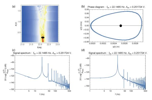
Figure 10: Typical measured system response around the linear system first mode at an excitation frequency  $f_{ex} \approx 22.15$  Hz and amplitude  $A_{ex} \approx 0.3925$  V. (a): density plot, the black oval represents the point of interest, (b): phase plot, the black circle shows the equilibrium point, (c): BSA displacement spectrum, (d): beam 1 displacement spectrum.
