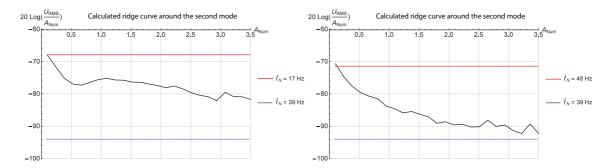
Figure 23: Calculated ridge curve of beam 1 displacement frequency response around the second mode for different BSA linear resonance. Left:  $f_N \approx 17$  Hz, right:  $f_N \approx 48$  Hz. The two horizontal lines correspond to the frequency response curve for the linear BSA: the continuous one is for the BSA frequency used in the non linear response while the discontinuous is the one obtained for the TMD.
