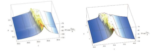
Figure 7: Surface plot of beam 1 displacement frequency response around the second mode. Left: measurement, right: model
