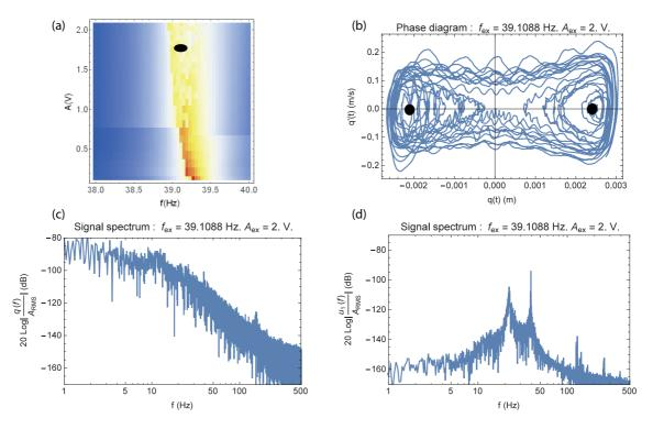
Figure 15: Typical measured system response around the linear system second mode at an excitation frequency  $f_{ex} \approx 39.11$  Hz and amplitude  $A_{ex} \approx 2$  V. (a): density plot, the black oval represents the point of interest, (b): phase plot, the black circles show the equilibrium points, (c): BSA displacement spectrum, (d): beam 1 displacement spectrum.
