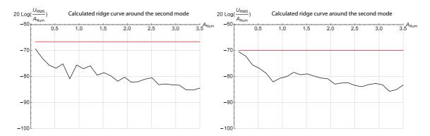
Figure 19: Calculated ridge curve of beam 1 displacement frequency response around the second mode for different BSA damping. Left: viscous damping  $\mu = 0.05$  kg/s, right: viscous damping  $\mu = 0.15$  kg/s. The straight line corresponds to the ridge curve for the linear BSA.
