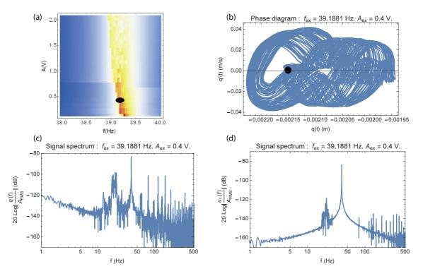
Figure 14: Typical measured system response around the linear system second mode at an excitation frequency  $f_{ex} \approx 39.19$  Hz and amplitude  $A_{ex} \approx 0.4$  V. (a): density plot, the black oval represents the point of interest, (b): phase plot, the black circle shows the equilibrium point, (c): BSA displacement spectrum, (d): beam 1 displacement spectrum.
