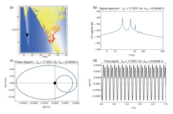
Figure 25: Computed BSA response. (a): density plot, the black oval represents the point of interest, (b): displacement spectrum, (c): phase plot, the black circle shows the equilibrium point, (d): displacement time recording.
