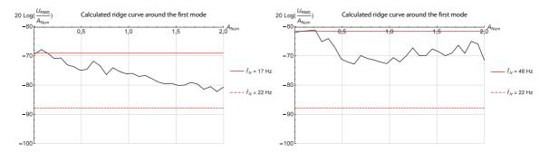
Figure 22: Calculated ridge curve of beam 1 displacement frequency response around the first mode for different BSA linear resonance. Left:  $\check{f}_N \approx 17$  Hz, right:  $\check{f}_N \approx 48$  Hz. The two horizontal lines correspond to the frequency response curve for the linear BSA: the continuous one is for the BSA frequency used in the non linear response while the discontinuous is the one obtained for the TMD.
