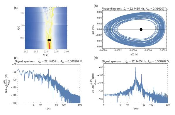
Figure 11: Typical measured system response around the linear system first mode at an excitation frequency  $f_{ex} \approx 22.15$  Hz and amplitude  $A_{ex} \approx 0.39$  V. (a): density plot, the black oval represents the point of interest, (b): phase plot, the black circle shows the equilibrium point,(c): BSA displacement spectrum, (d): beam 1 displacement spectrum.
