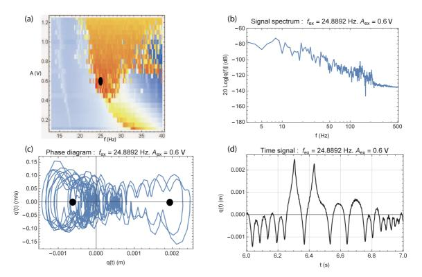
Figure 26: Measured BSA response. (a): density plot, the black oval represents the point of interest, (b): displacement spectrum, (c): phase plot, the black circles show the equilibrium points, (d): displacement time recording.
