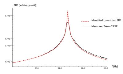
Figure 5: Example of linear modal identification. The black continuous curve represents experimental FRF of beam 2. The red discontinuous curve represents the identified Lorentzian with frequency  $f_1^e = 22.2 - i0.006$  Hz
