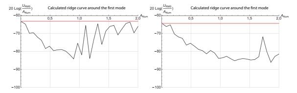
Figure 17: Calculated ridge curve of beam 1 displacement frequency response around the first mode for different BSA damping. Left: viscous damping  $\mu = 0.05$  kg/s, right: viscous damping  $\mu = 0.15$  kg/s. The straight line corresponds to the ridge curve for the linear BSA.
