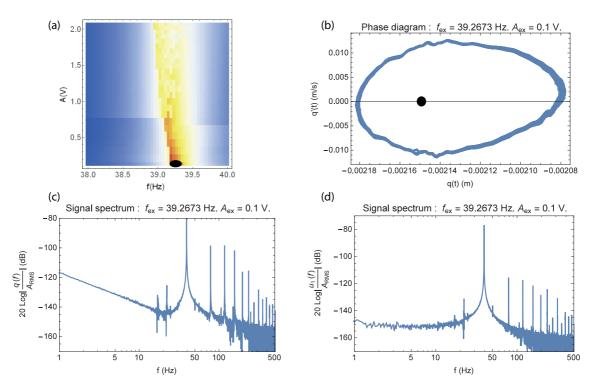
Figure 13: Typical measured system response around the linear system second mode at an excitation frequency  $f_{ex} \approx 39.27$  Hz and amplitude  $A_{ex} \approx 0.1$  V. (a): density plot, the black oval represents the point of interest, (b): phase plot, the black circle shows the equilibrium point, (c): BSA displacement spectrum, (d): beam 1 displacement spectrum.
