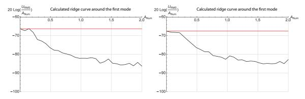
Figure 18: Calculated ridge curve of beam 1 displacement frequency response around the first mode for different BSA damping. Left: viscous damping  $\mu = 0.35$  kg/s, right: viscous damping  $\mu = 0.50$  kg/s. The straight line corresponds to the ridge curve for the linear BSA.
