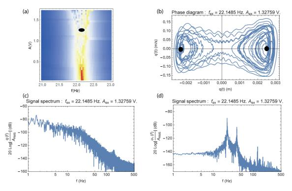
Figure 12: Typical measured system response around the linear system first mode at an excitation frequency  $f_{ex} \approx$  22.15 Hz and amplitude  $A_{ex} \approx 1.33$  V. (a): density plot, the black oval represents the point of interest, (b): phase plot, the black circles show the equilibrium points,(c): BSA displacement spectrum, (d): beam 1 displacement spectrum.
