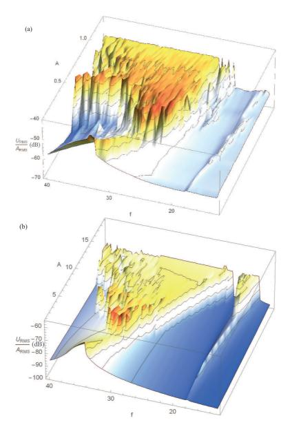
Figure 4: Frequency response of the RMS value for the measured (a) and computed (b) BSA displacement  $20 \log(\tilde{q}_{RMS}/A_{RMS})$  vs frequency and amplitude. On both curves, the thin black curves are separated by 5 dB.
