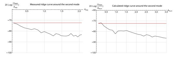
Figure 9: Ridge curve of beam 1 displacement frequency response around the second mode. Left: measurement, right: model. The straight line corresponds to the ridge curve for the linear BSA.
