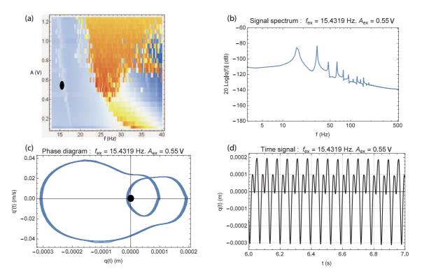
Figure 24: Measured BSA response. (a): density plot, the black oval represents the point of interest, (b): displacement spectrum, (c): phase plot, the black circle shows the equilibrium point, (d): displacement time recording.
