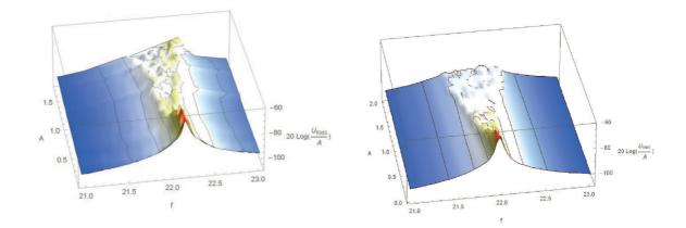
Figure 6: Surface plot of beam 1 displacement frequency response around the first mode. Left: measurement, right: model
