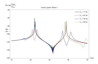
Figure 21: Four computed beam 1 different linear frequency responses. Each curve corresponds to the BSA acting as a linear absorber with a particular resonance frequency: 17 Hz, 22 Hz (TMD for the first mode), 39 Hz (TMD for the second mode) and 48 Hz and viscous damping  $\mu = 0.24$  kg/s.
