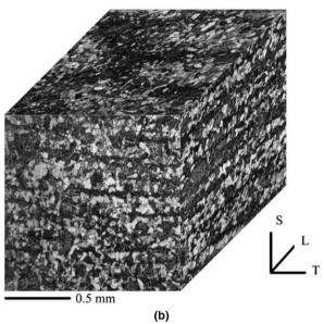
Fig. 1. (a) Microstructure of the low alloyed steel A508 revealed by a Stead le Chatelier solution and (b) the banded structure.
