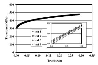
Fig. 9. Effect of a Gaussian random noise on a theoretical tensile curve simulated using the parameters K = 250, a = 1.3 and m = 0.29. The result is illustrated for different perturbed theoretical tensile curves. For the sake of clarity, only four curves out of 10000 are plotted.
