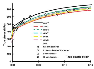
Fig. 4. True stress–true strain tensile curves obtained for the different orientations and sampling locations (core, inner and outer skin of the piece of vessel) and the stress–strain correlations obtained by ball indentation testing with various indenter radii.
