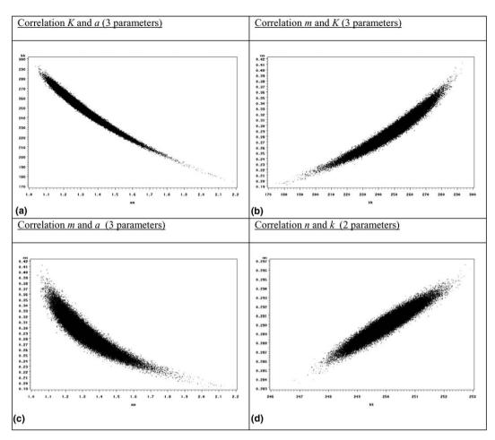
Fig. 10. Correlations existing between the different parameters estimated by the SAS software for the 10000 perturbed theoretical curves: (a)–(c) correspond to correlations between the three parameters related to Ludwik Hollomon's law while (d) corresponds to the correlation between the two parameters of Hollomon's law.
