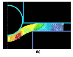
Fig. 2. (a) Schematic representation of the small-punch test jig and (b) of the FORGE2 configuration for simulation without clamping.
