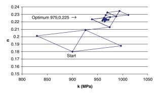
Fig. 8. Illustration of the different steps of the simplex optimization obtained by applying our algorithm to determine the optimal parameters of the Hollomon constitutive law with respect to a FEM of a small-punch test.
