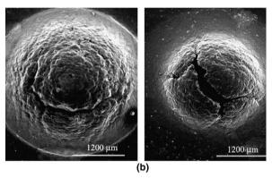
Fig. 7. (a) Influence of the thickness of the sample on the energy value calculated from a small-punch test curve and (b) example of fractured samples having a 0.6 mm thickness (left view) and 0.15 mm thickness (right view).
