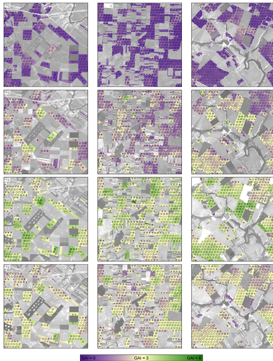
Figure 15: Spatial comparison between high spatial resolution GAI maps from SPOT (in the background) with MODIS GAI estimations (dots) for 3 different 7.2 \times 7.2 km zones at the following days of year (from top to bottom): 76, 102, 123 and 144. The size of the dots relates to the pixel purity of the MODIS estimations, with larger dots being purer than smaller ones (only estimations above 75% pixel purity are shown). The images in the background are the respective Red channel of the original SPOT imagery used to derive the GAI maps.
