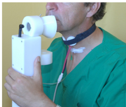
Fig. 3. EVA aerophonometer to record simultaneously the speech, airflows and pressure. Additional devices can be added as EGG (right picture).
