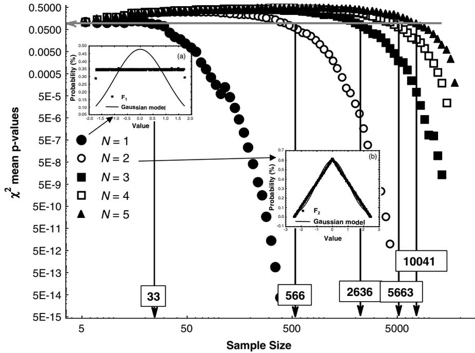
Fig. 1. Evolution of the  $\chi^2$  mean  $p$ -values as a function of the sample size  $n$  for a degree of summation  $N$  varying from 1 to 5. The corresponding distributions  $F_N$  are inserted in windows as well as the result of their Gaussian modelling for  $N = 1$  and  $N = 2$ .
