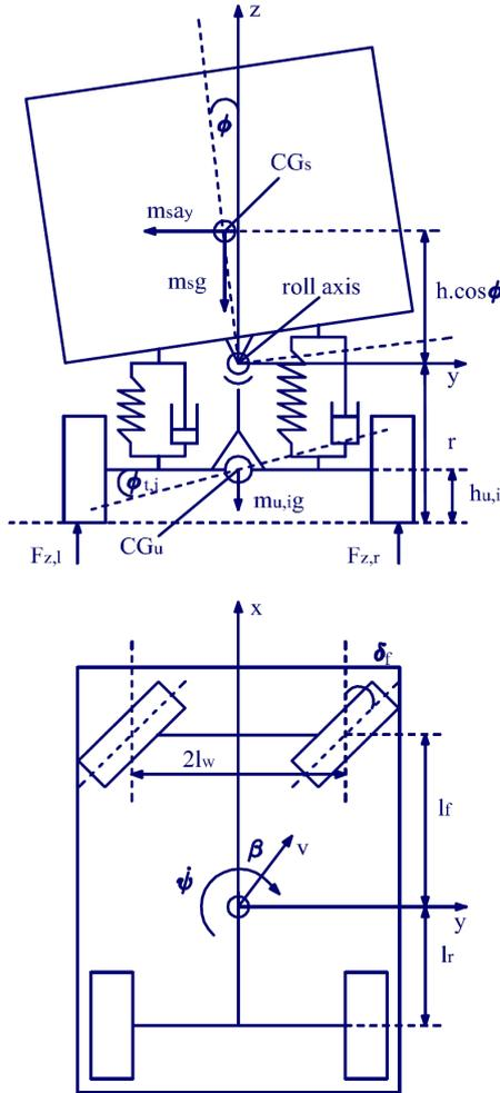
Fig. 2. Yaw-Roll model of single unit heavy vehicle.
