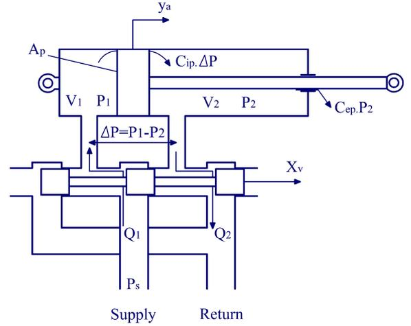
Fig. 1. Diagram of the electronic servo valve hydraulic damper.
