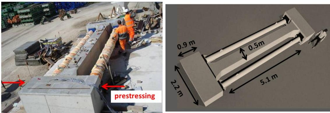
Figure 1: Geometry of the RG specimens
