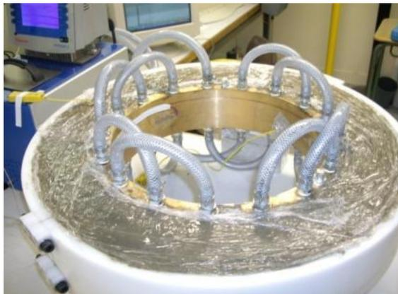
Figure 12 : Active test ring with its mould
