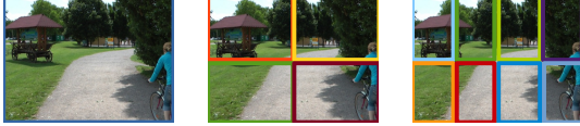
Fig. 3. From left to right, windows are constructed from the root window by splitting it iteratively. The proposal tree follows the structure and color code of Fig. 1.
